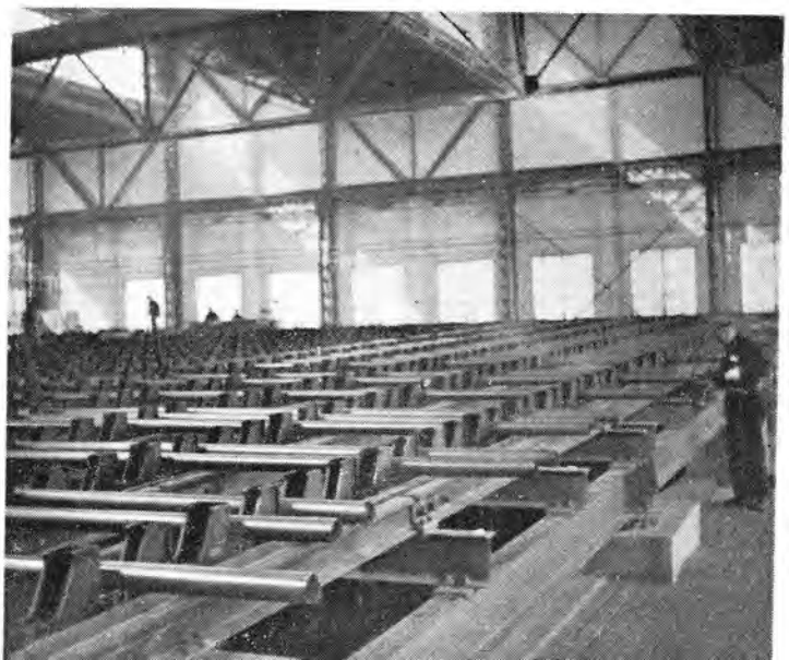
Seamless tubes in the cooling shop
